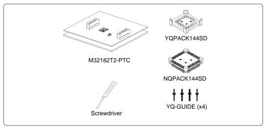
Figure 1 Package components of the M32182T2-PTC
